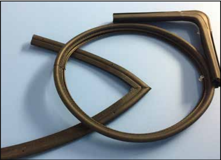
Cut, Mitered and Bonded
